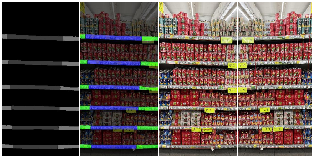
Figure 4. Sample of predicted mask and the corner point detection result.
